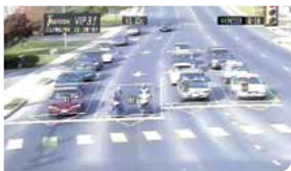
Vehicle presence detection at intersections
