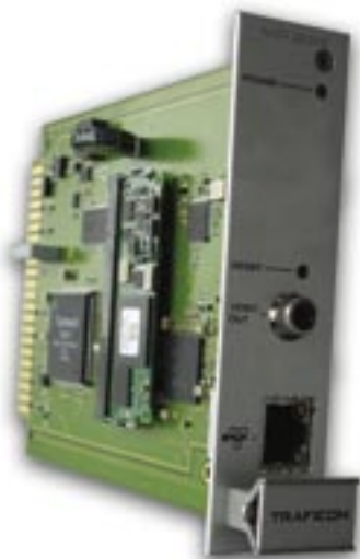
The Traficon VIP BIKE detector board
