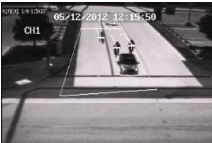
Thermal cameras can consistently differentiate bicycles from other traffic.
