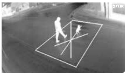
On-crossing pedestrian detection
